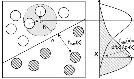
Figure 3.4: Demonstration of computing  $f(x)$  by the PP classifiers. Left: SVM-based PP tries to find the decision boundary  $w$ . Right: 1-D visualization of the  $+1/-1$  densities (dark circles for  $+1$  and white circles for  $-1$ ). KDE-based PP measures  $f_{\text{kde}}(x) = d^+(x)/d^-(x)$  where  $d$  is estimated with a neighborhood of  $h$ .
