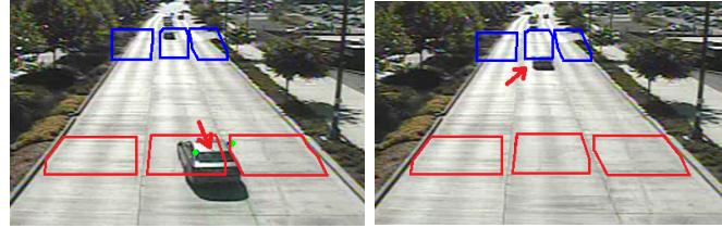
Figure 2.7: Step-by-step process of mapping traffic flow. Left: a vehicle entering the entry box. Right: a vehicle entering the exit box.
