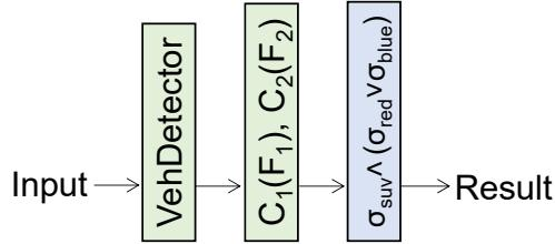
Figure 4.2: Query plan for retrieving  $(\text{Red} \vee \text{Blue}) \wedge \text{SUV}$  from traffic videos, where VehDetector is a DNN-based vehicle detector,  $F_1$ ,  $F_2$  and  $C_1$ ,  $C_2$ , are feature extractors and classifiers respectively, to extract the color and type for each detected vehicle.
