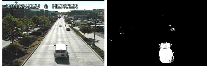
Figure 2.8: Background subtraction. Left: a vehicle entering the camera view. Right: binary mask indicating moving objects.
