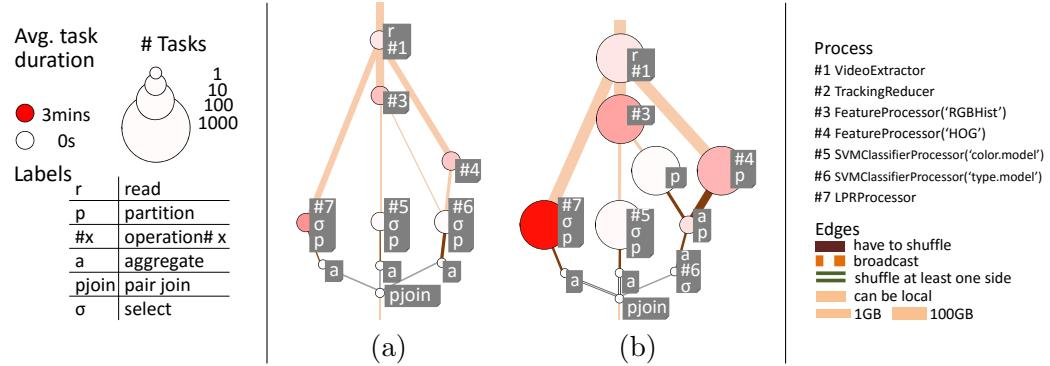
Figure 2.5: Dataflow and query plans of Amber Alert for (a) 1 GB input and (b) 100 GB video input. Note that the 100 GB input automatically parallelizes the tasks to minimize the query plan cost and the query latency. The workload is distributed nicely among the cluster nodes; partition and aggregation happen according to different input sizes.
