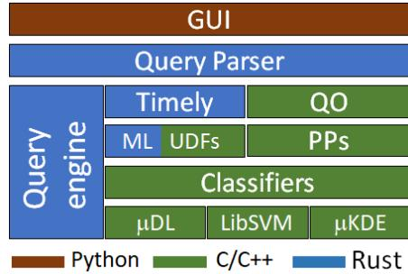
Figure 4.1: A cross-platform, data-parallel engine for DNN-enabled ML. User query: Standard SQL + UDF syntax. See [81]. Timely Dataflow: Rust implementation of Naiad [9]. Query engine: Join node, filter logic, columnar store for blobs etc.  $\mu$ DL: A light-weight DNN engine in C/C++.  $\mu$ KDE: A Kernel Density Estimator in C/C++.
