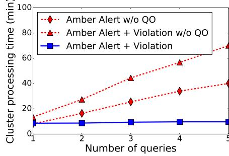
Figure 2.13: As the number of queries scale, query optimization ensures that the cluster processing time for both sets of queries stays constant by using auto-parallelization and de-duplication.
