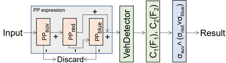
Figure 4.4: Modified query plan with PPs for retrieving  $(\text{Red} \vee \text{Blue}) \wedge \text{SUV}$  from traffic videos.
