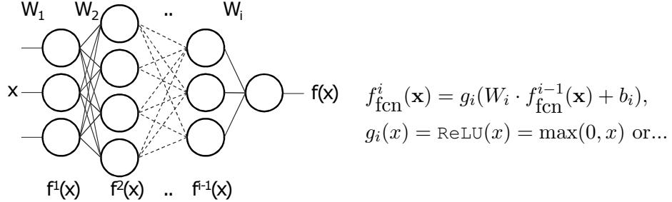
Figure 3.6: Left: structure of a fully connected neural network.  $W_i$  are different fully connected layers. Right: formula at layer  $i$ . The input  $f_{\text{fcn}}^0(\mathbf{x}) = \mathbf{x}$ .
