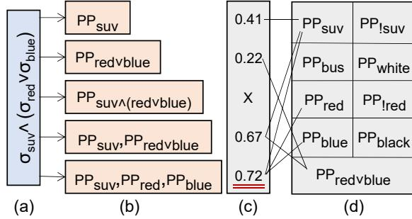
Figure 4.3: Demonstration of the query optimization process in our system. (a) Input complex predicate. (b) Candidate PP expressions that are implied by the original predicate. (c) Estimated data reduction rate for each PP expression while satisfying accuracy threshold: ‘X’ indicates no matching PP in corpus. We underline the expression that has the largest data filtering rate. (d) Corpus of available PPs.
